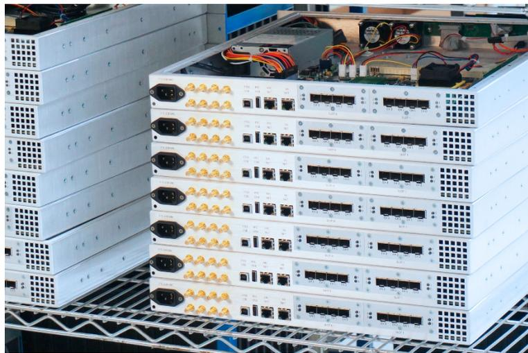
**Figure 4:** Assembled ROACH (reconfigured, open architecture, computing hardware) systems make observation and analysis of deep space and our universe possible.
